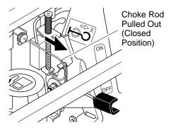
Figure 20 - Choke Rod Closed (Model RGH3000PR Only)
